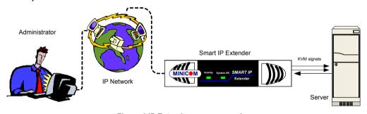
Figure 1 IP Extender usage scenario
